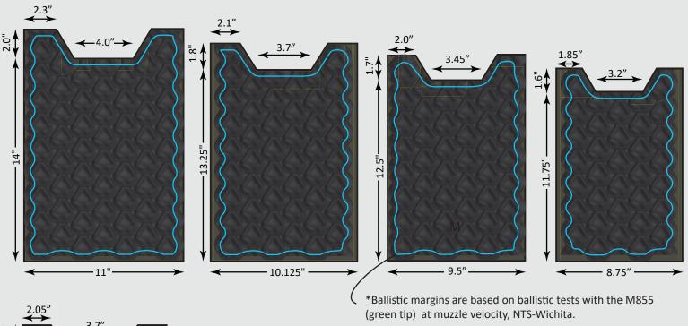
Ballistic panels are encased in water-tight nylon covers. Dimensions are ±0.25". Panel thickness is 1.2".
