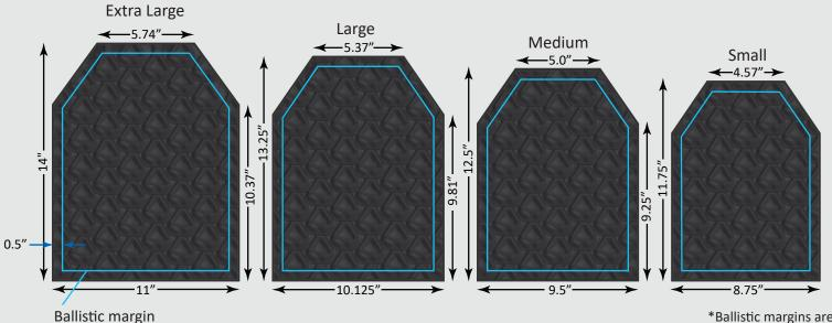
Ballistic panels are in watertight nylon covers. Length and width dimensions are ±0.25". Panel thickness is 1.2"
