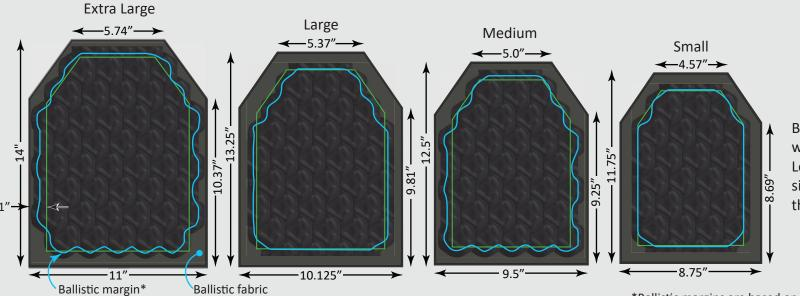
Ballistic panels are in a water-tight nylon cover. Length and width dimensions are ±0.25". Panel thickness is 1.2"
